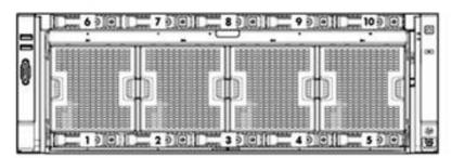
1-10 Ten (10) SFF Hot-plug HDD/SSD drive bays NOTE: Drives installed in bays 6-10 require the optional SAS backplane kit. NOTE: Optional NVMe drives are only supported in Drive bays 6-10.
