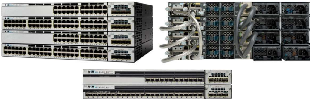
Figure 1. Cisco Catalyst 3750-X Series Switches (Front and Back)
